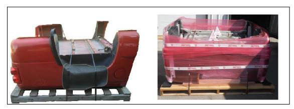
It is not recommended that you ship a pickup box via an LTL carrier due to the high probability of damage during shipment. However, should this be unavoidable, it is recommended that you build a perimeter around the outside that looks like a 78"x78"x48" wooden box, then stretch wrap it.
