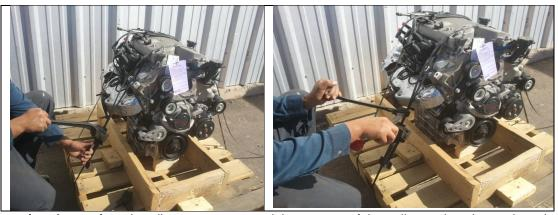
**Securing the engine -** banding must go around the runners of the pallet not just the top boards and should go from one runner, over the part, then around the other runner and back over the part. The banding should form a double "U" over the part, not a circle around it. This forms a secure hold that is not subject to damage by fork lift forks or other lifting equipment that can cause the banding to loosen or break.
